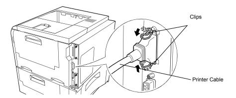
3. Plug the other end of the printer cable into the computer's parallel (Centronics) interface connector. This connector is usually marked PRINTER. For details, please refer to the hardware manual for the computer.
